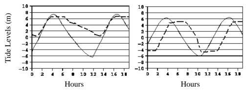
Figure 2. Indicative Upstream (dashed) and Downstream (solid) Water levels for ebb (left) and ebb and flood (right) modes of operation
